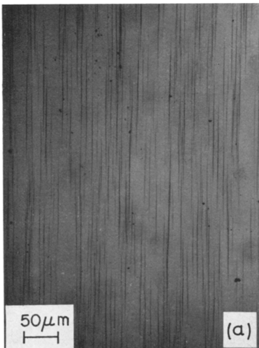
Figure 6 Crazes formed at 78° K in a PMMA specimen with a continuously varying gauge width, viewed in transmitted light: (a) original external surface; (b) cross section. Note the depth of craze penetration decreases with decreasing stress. Stress axis horizontal.
